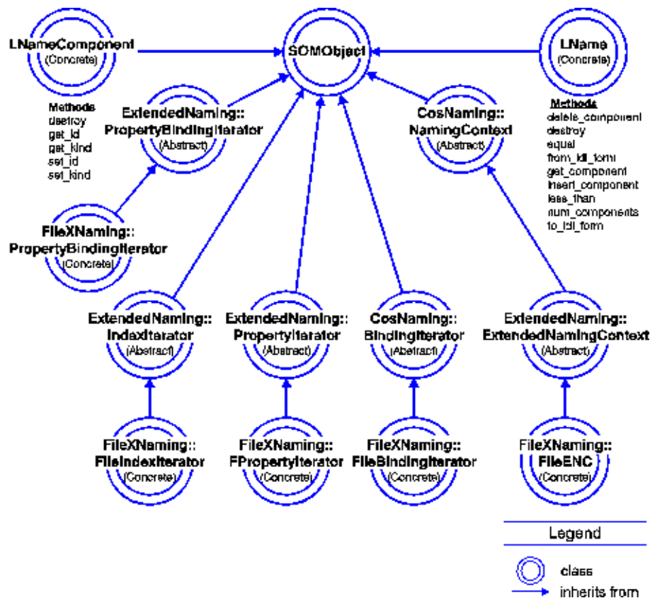
Figure 4. Derivation for SOMObjects 3.0 Naming Service, Part Two
